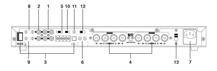
**1. Main Input/Output:** The DAC-XX200 Main Input consists of stereo RCA jacks and are used as the amplifier's primary audio inputs. The Main Output also consists of stereo RCA jacks and can passthrough the DAC-XX200's Main Input audio signal to another amplifier.
