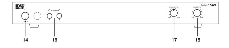
**14. Power Switch:** The front-panel Power Switch turns the XX200 on or off. A red LED indicates connection to AC power while in standby mode and turns green indicating audio signal is present.
