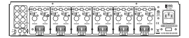
Connect the right or left output from the audio source to the right or left input of the zone you are bridging. Repeat this for each zone you want in bridged mode.
