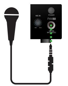
Step 1: Turn the Mic In volume knob down (counter-clockwise) to the "Min" position.
