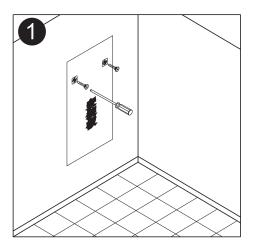
Using the supplied hardware install the 2 mounting screws into the desired mounting location.
