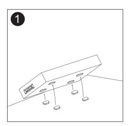
Install the supplied non slip feet to the back of the cabinet.
