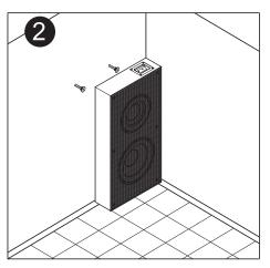
Line up the mounting screws with the mounting slots on the back of the SL800 and install.
