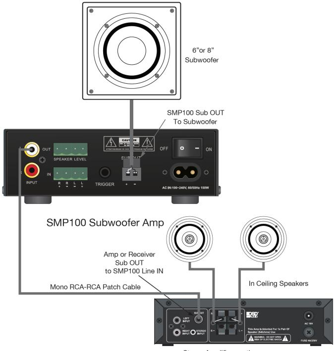
Stereo Amplifier or other amp/receiver with a subwoofer out
